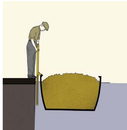
The toll clerk measured how high the boat is in the water using a gauging rod.
